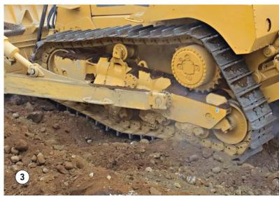
Positive Pin Retention Sealed and Lubricated Track
